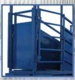
The main gate at the top keeps loaded livestock from running back off the trailer while the secondary gate closes the opening at the side.
