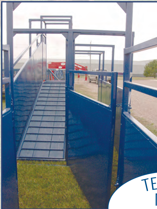
Y splitter diverting cattle to Loading Chute
